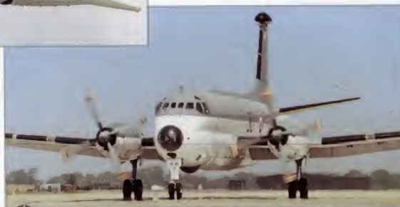
Above: One of Germany's Atlantics shows its retracted radar radome and sonobuoy launch tubes.
